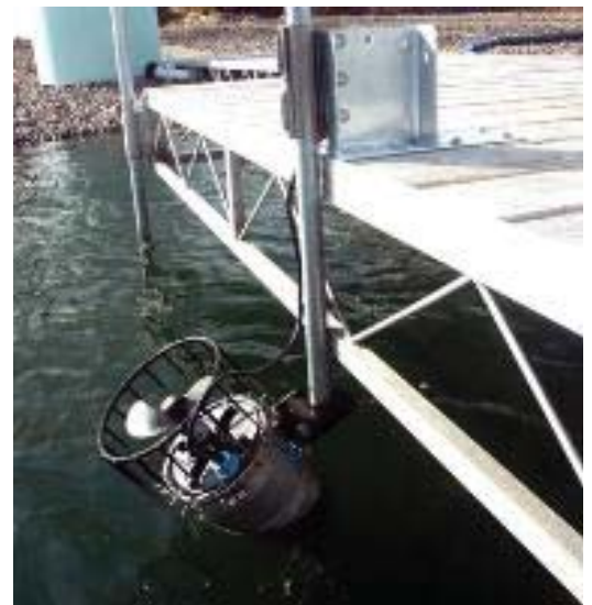
Figure 5.5 Kasco Circulator with Dock Mount $1000 1hp unit, 120 - 240V, circulates 30m highly efficient, low power consumption vertical and angled mounting * image portrays a dock mounted circulator, the circulator for Trout Lake would make use of the dock mount on a steel post in the water *consider reconfiguring the motors to run with solar energy through the use of solar panels
