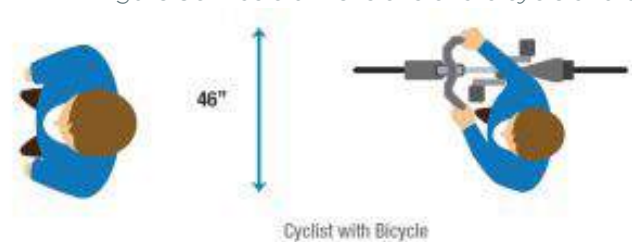
Figure 30: Basic dimensions of a bicycle and cyclist
