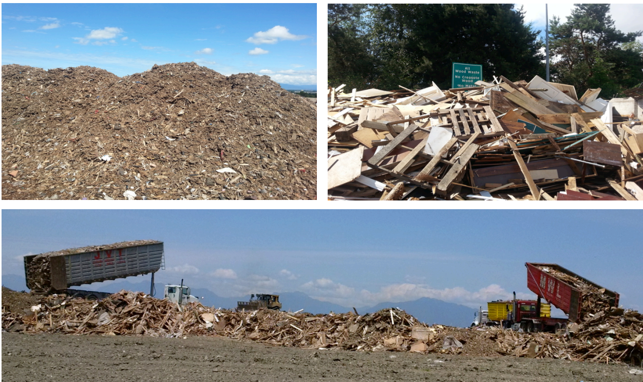
Figure 13 Demo Hog (Wood Fines <math>< 3'' \times 3''</math>), the Top Left Picture and Mixture of Tread/Painted Wood Waste, the Top Right and Bottom Pictures
