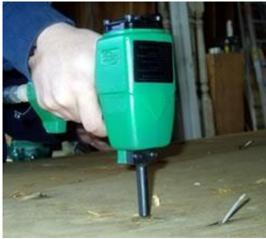
Figure 9 A pneumatically-powered de-nailer tool
