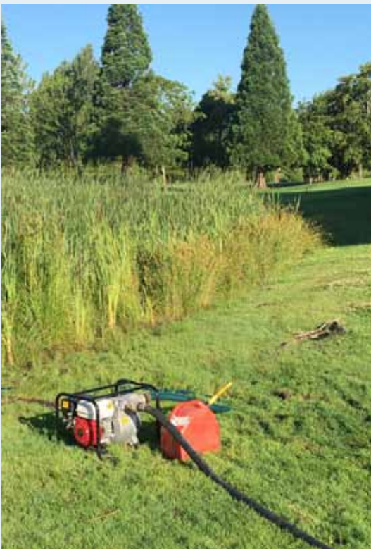
The pump at left is a stopgap solution to prevent flooding while waiting for a debris blasting service. The drain at right is not protected and requires daily clearing of debris to prevent clogging. photo credit: Jennifer Rae Pierce
