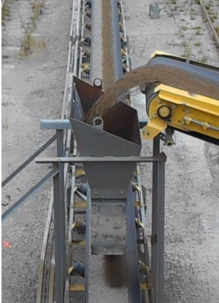
Figure 7: Blending rubble with mineral aggregate for backfill (Photo courtesy of Kent Yard)
