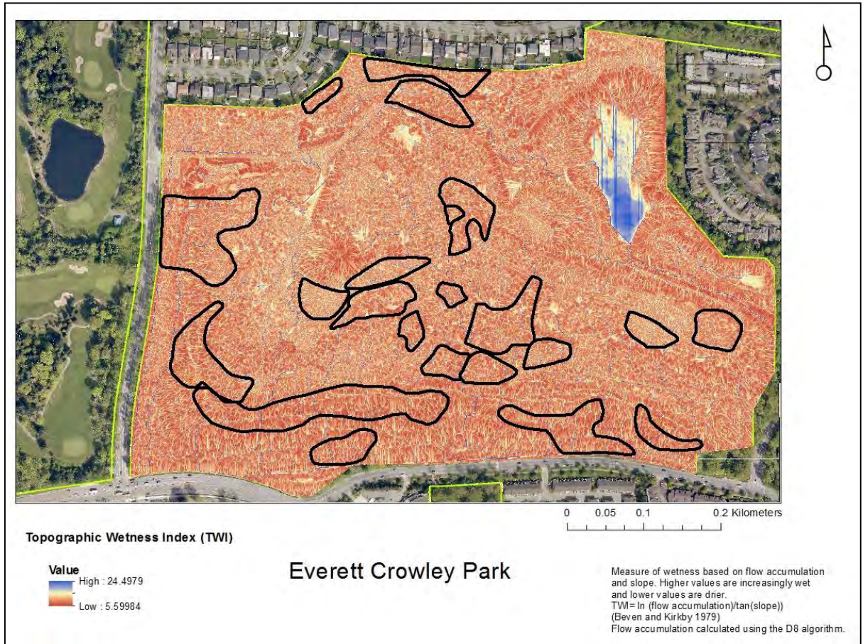
TWI map for ECP. Outline of current and proposed restoration sites shown. . Refer to map on page 30 for associated names
