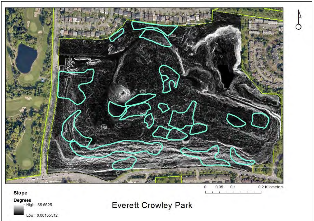
Slope map for ECP. Outline of current and proposed restoration sites shown. Refer to map on page 30 for associated names
