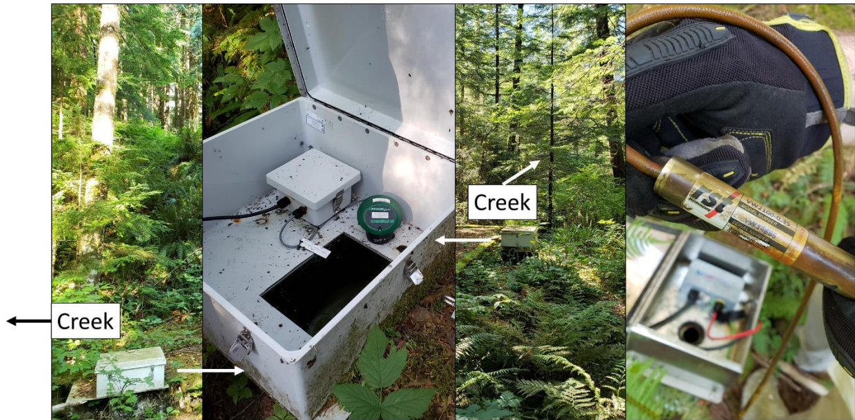
Figure 1 – Seymour Dam: Monitoring instruments for creeks (first th); Vibe wire for piezometer in wells (fourth)
