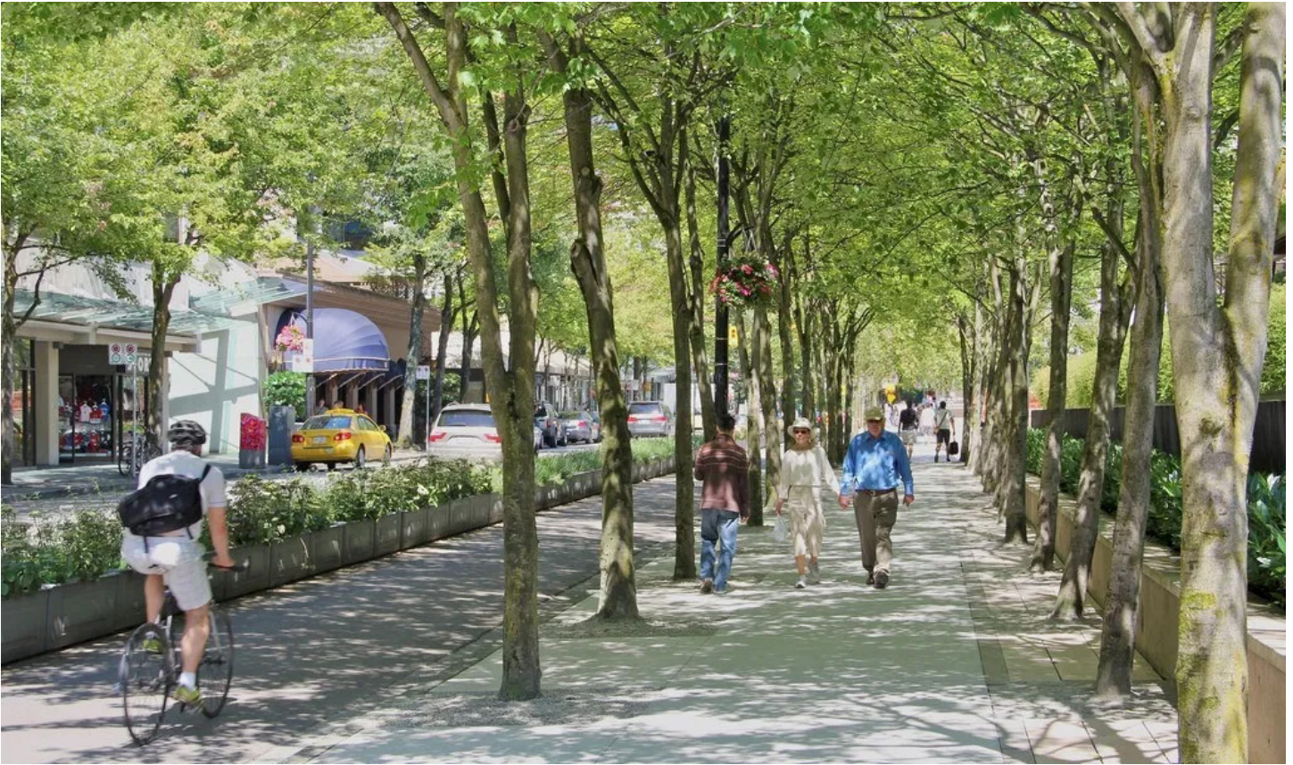
Tree canopy and green street design features can improve pedestrian comfort by providing shade and protection from the elements. Green design features also have the potential to reduce surface water runoff by increasing the amount of effective pervious area, as well as mitigating the urban heat island effect common to many cities. Image by Paul Krueger via flickr.
