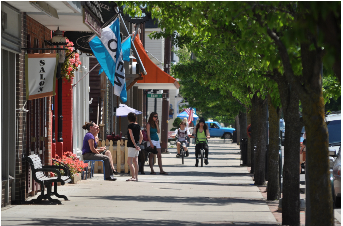
Increasing footpath width creates a more comfortable amount space for pedestrians to pass one another and walk side-by-side. Sidewalk trees can also serve to improve pedestrian experience by providing shade and some degree of weather protections, as well as providing a partial screen from adjacent traffic. Image by Michigan Municipal League via BetterBurb .
