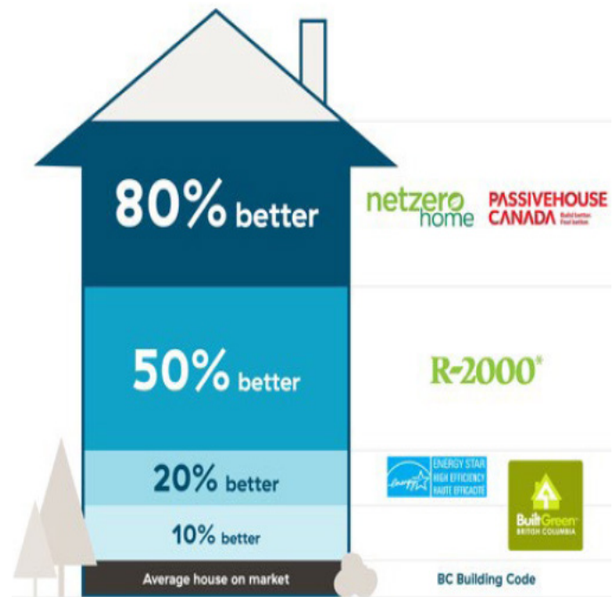
Standards for energy-efficiency in new homes, from “Energy Efficiency for First Nation Housing Managers,” Pinna Sustainability, n.d.
