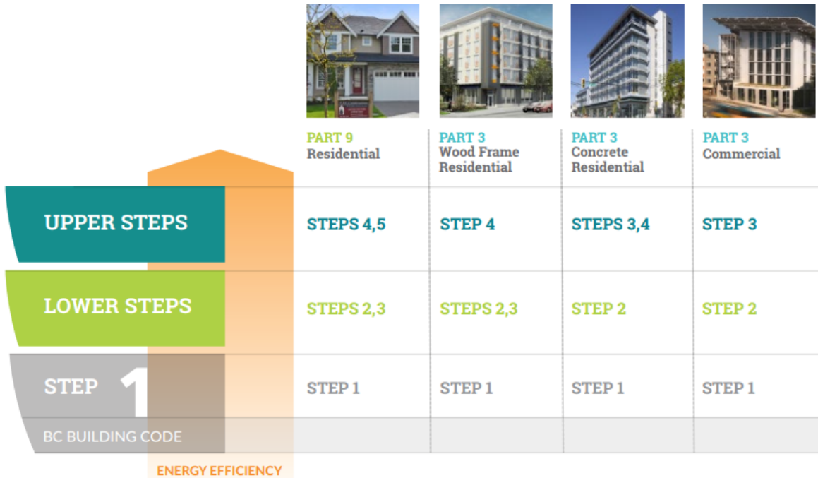
Figure 4. Definition of Lower and Upper Steps by building type (Part 9 and Part 3) [5]
