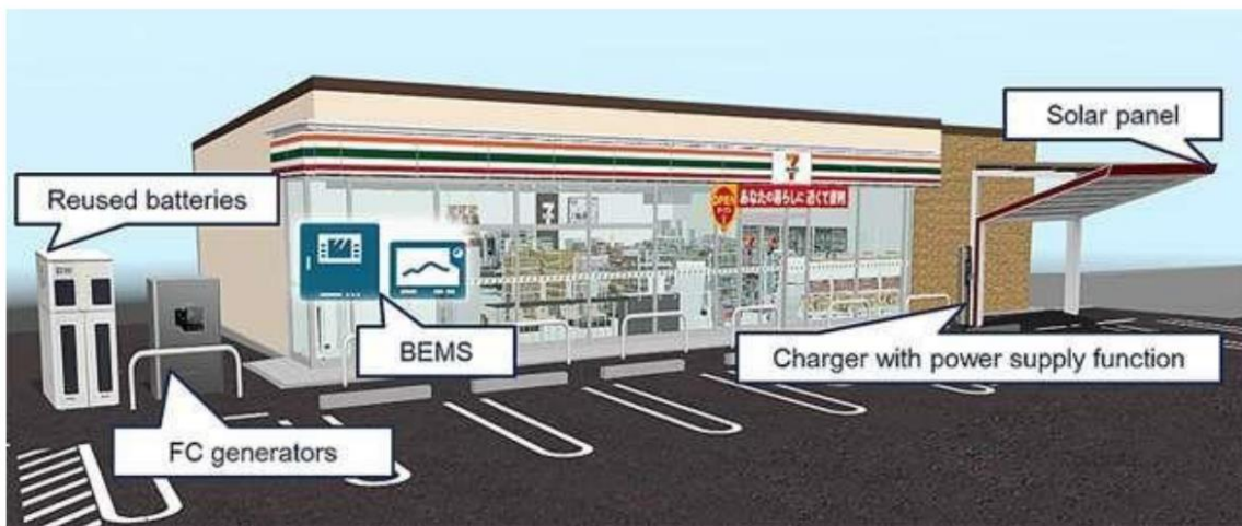
Figure 2: Reused Electric vehicle batteries Power a 7-11 Store in Japan 23
