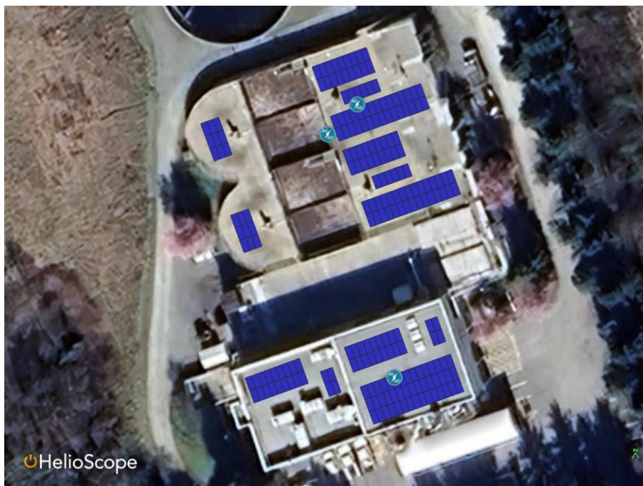
Figure 18: Rooftop solar PV system designed atop Saanich Peninsula WWTP
