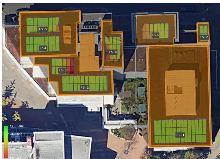
Figure 26: Solar PV system shading heatmap (CRD HQ)
