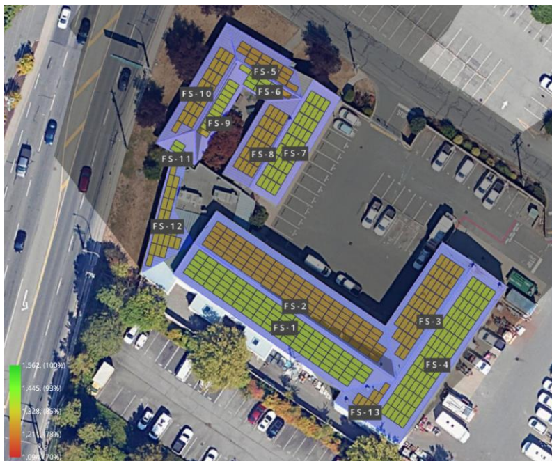
Figure 35: Solar PV system shading heatmap (IWS HQ)
