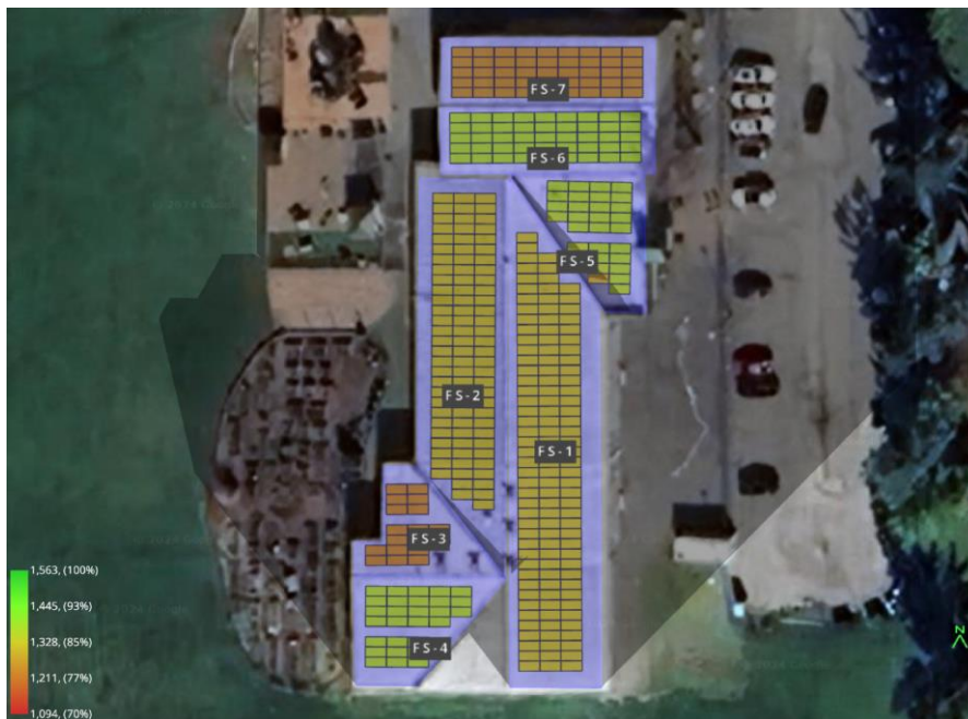
Figure 32: Solar PV system shading heatmap (Greenglade CC)
