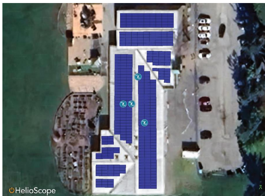
Figure 30: Rooftop solar PV system designed atop Greenglade Community Centre
