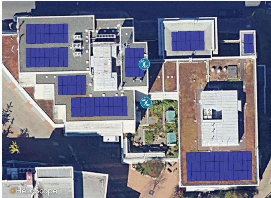
Figure 24: Rooftop solar PV system designed atop CRD HQ
