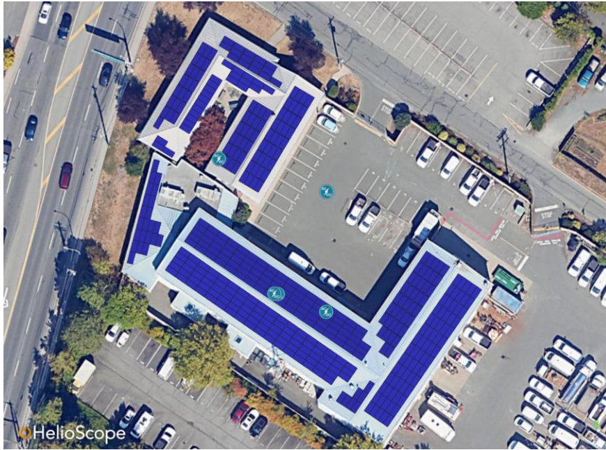
Figure 33: Rooftop solar PV system designed atop IWS HQ
