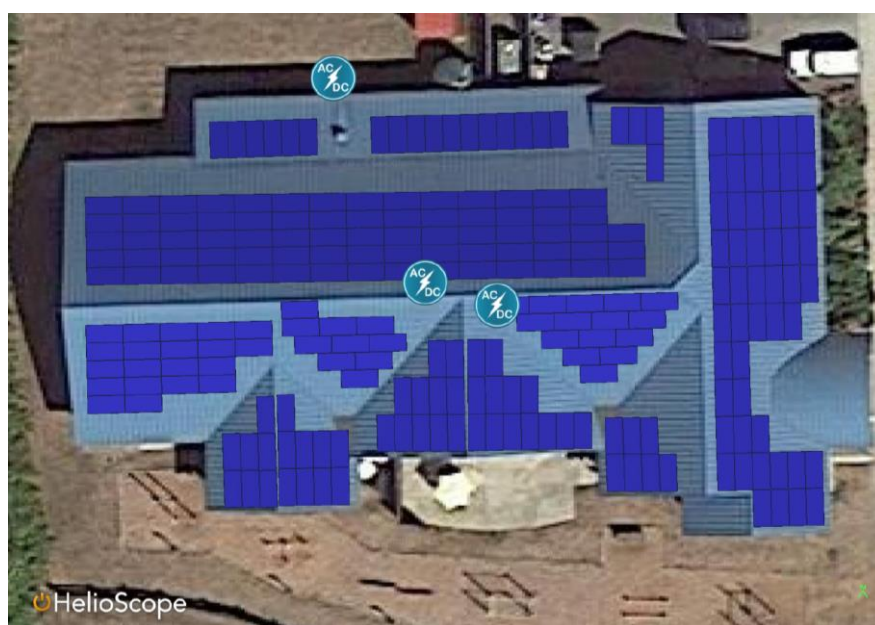
Figure 21: Rooftop solar PV system designed atop Rainbow Road Aquatic Centre
