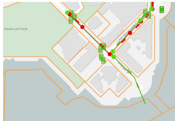
Figure 4-2 Stormwater runoff disposal into False Creek using Gravity system from the Richard Street segment
