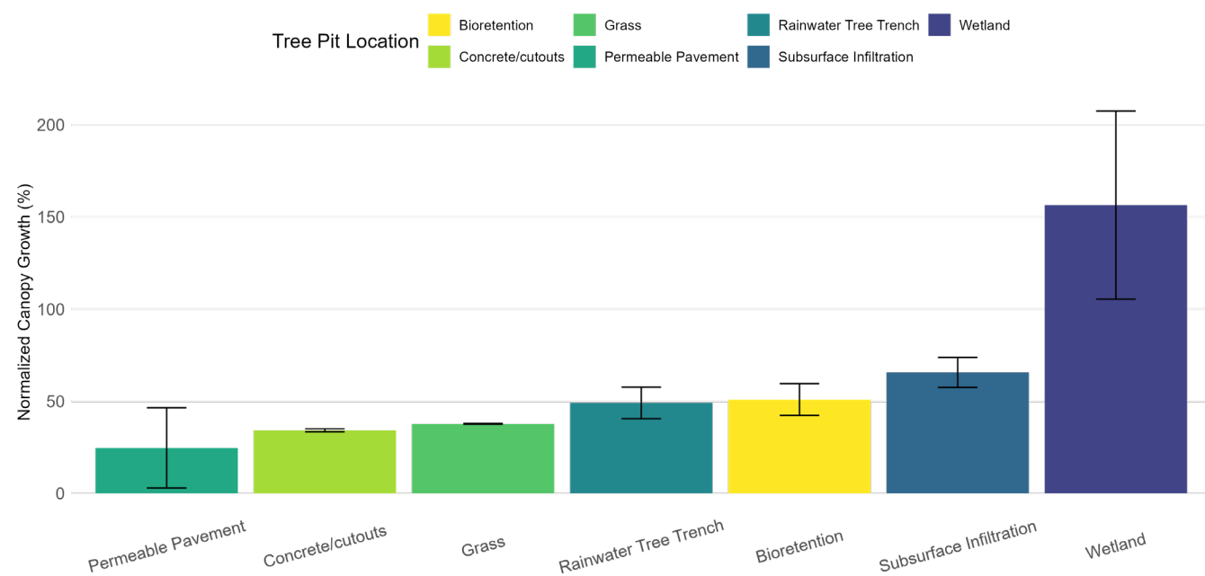
Figure A.4: Mean 2018-2022 normalized canopy growth (%) by tree pit locations. Error bars represent mean \pm 1 standard error.
