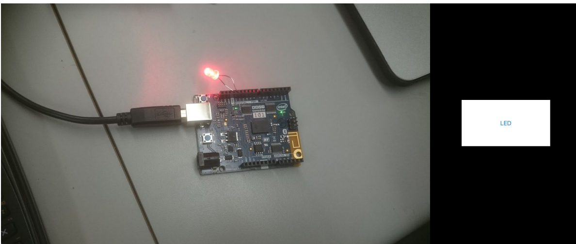
Figure 3.1 - Bluetooth Connection LED is shown High
