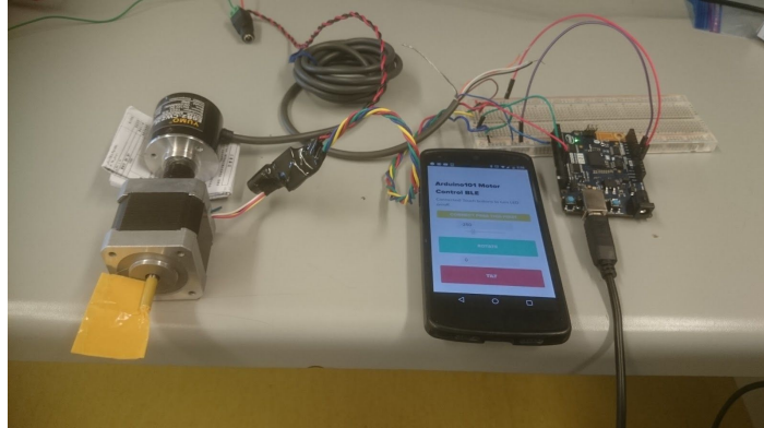
Figure 2.1 - Motor Control System
