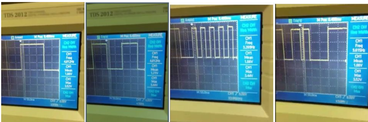
Figure 2.3 - Variable frequency output from microcontroller
