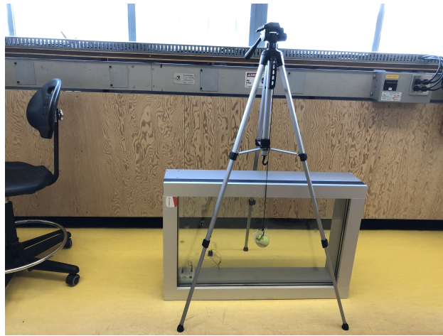
Figure E1: The system setup for the system reliability test. The accelerometer is placed in an appropriate location on the window.
