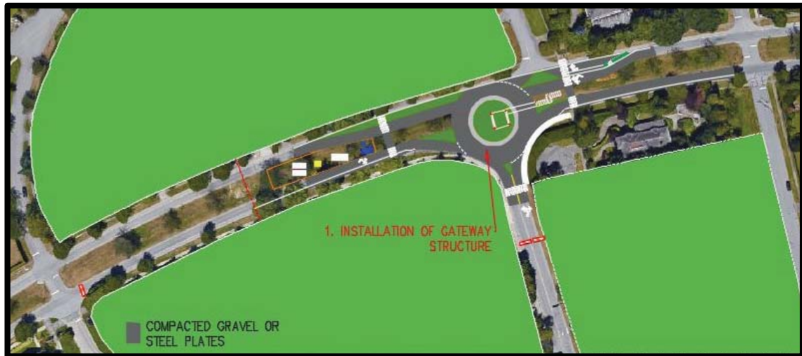
Figure 16 - Stage 11: Gateway Installation
