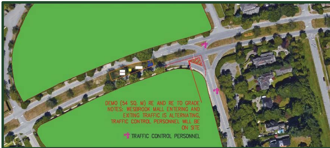
Figure 6 - Stage 2: Southwest Island Demolition
