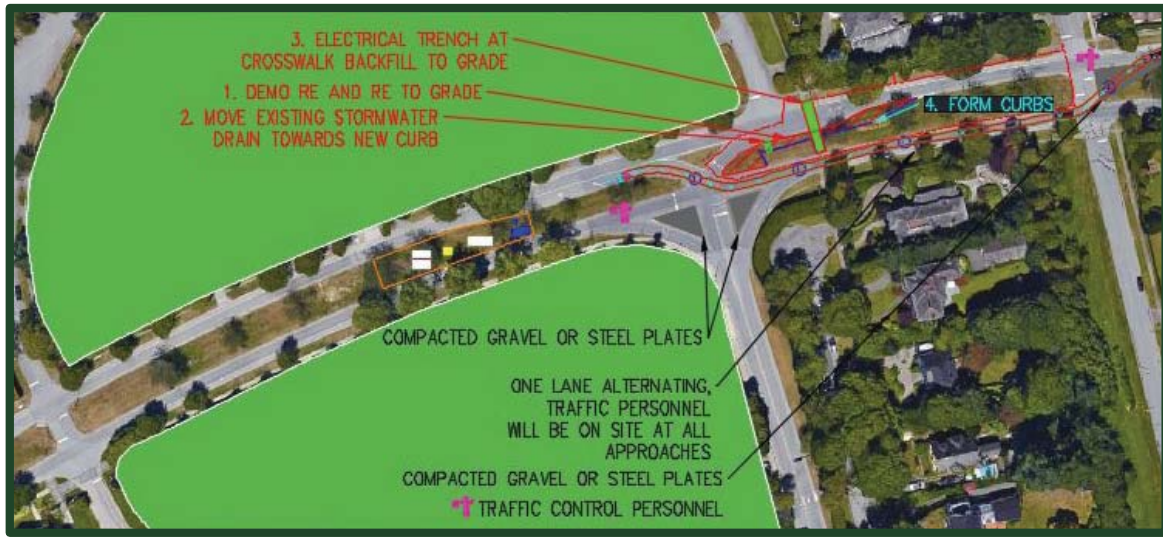
Figure 9 - Stage 4: East Median Demolition
