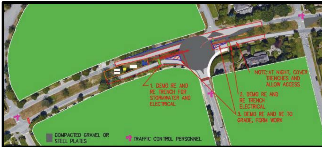
Figure 13 - Stage 8: Electrical Trenching
