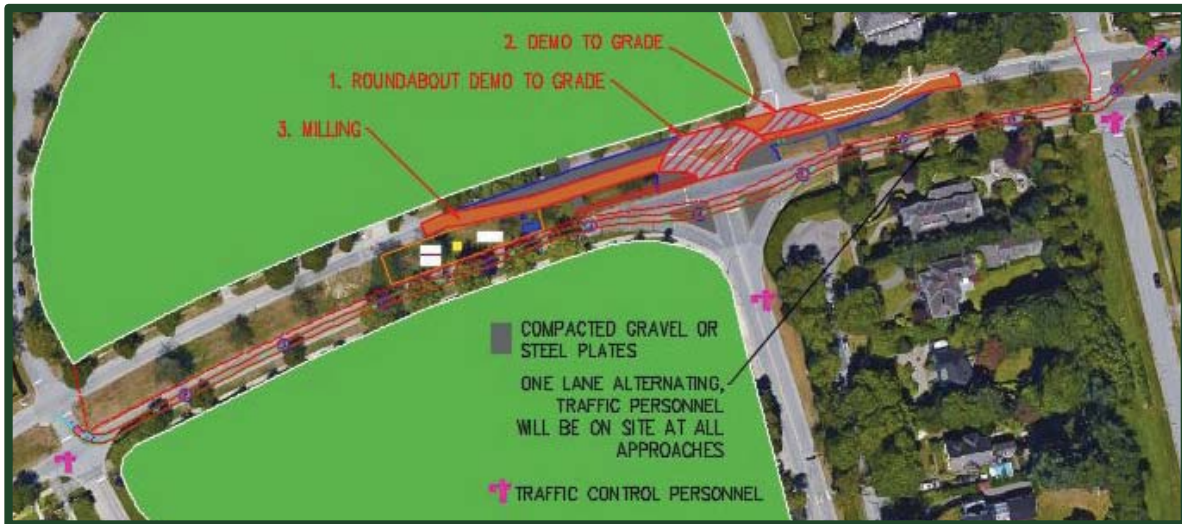
Figure 11 - Stage 6: Northern Roundabout Construction
