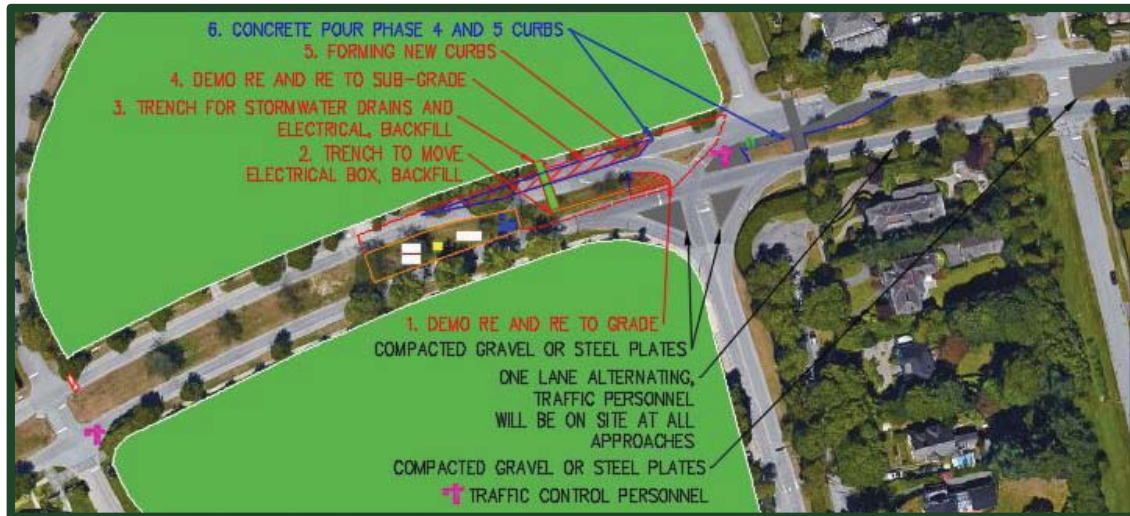
Figure 10 – Stage 5: West Median Demolition and Northwest Island Construction
