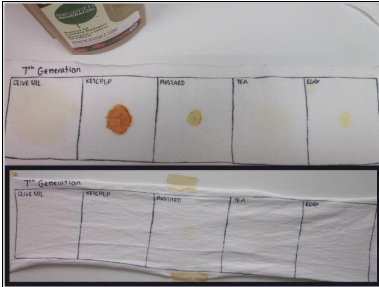
Figure 7. Seventh Generation before and after performance testing
