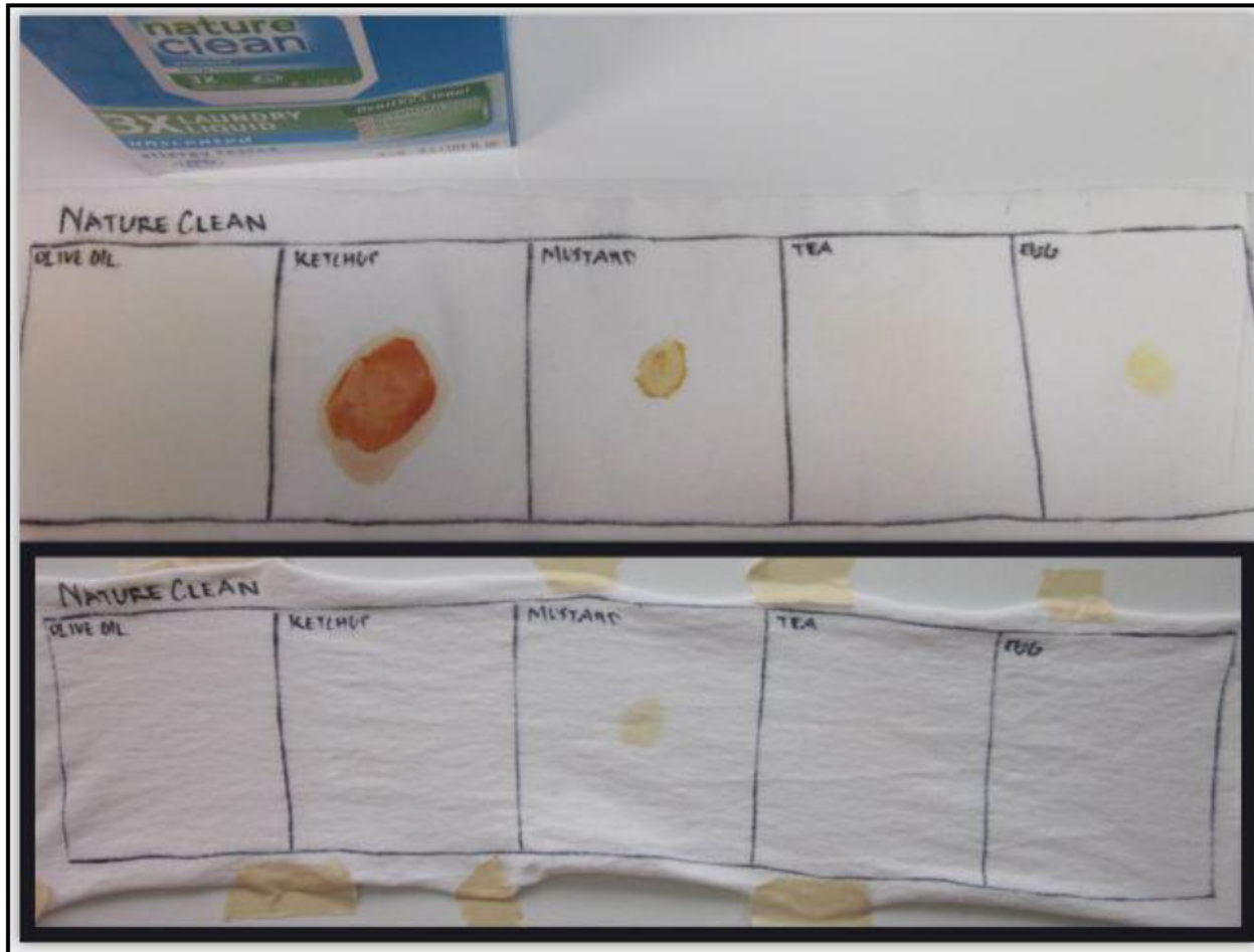
Figure 9. NatureClean before and after performance testing
