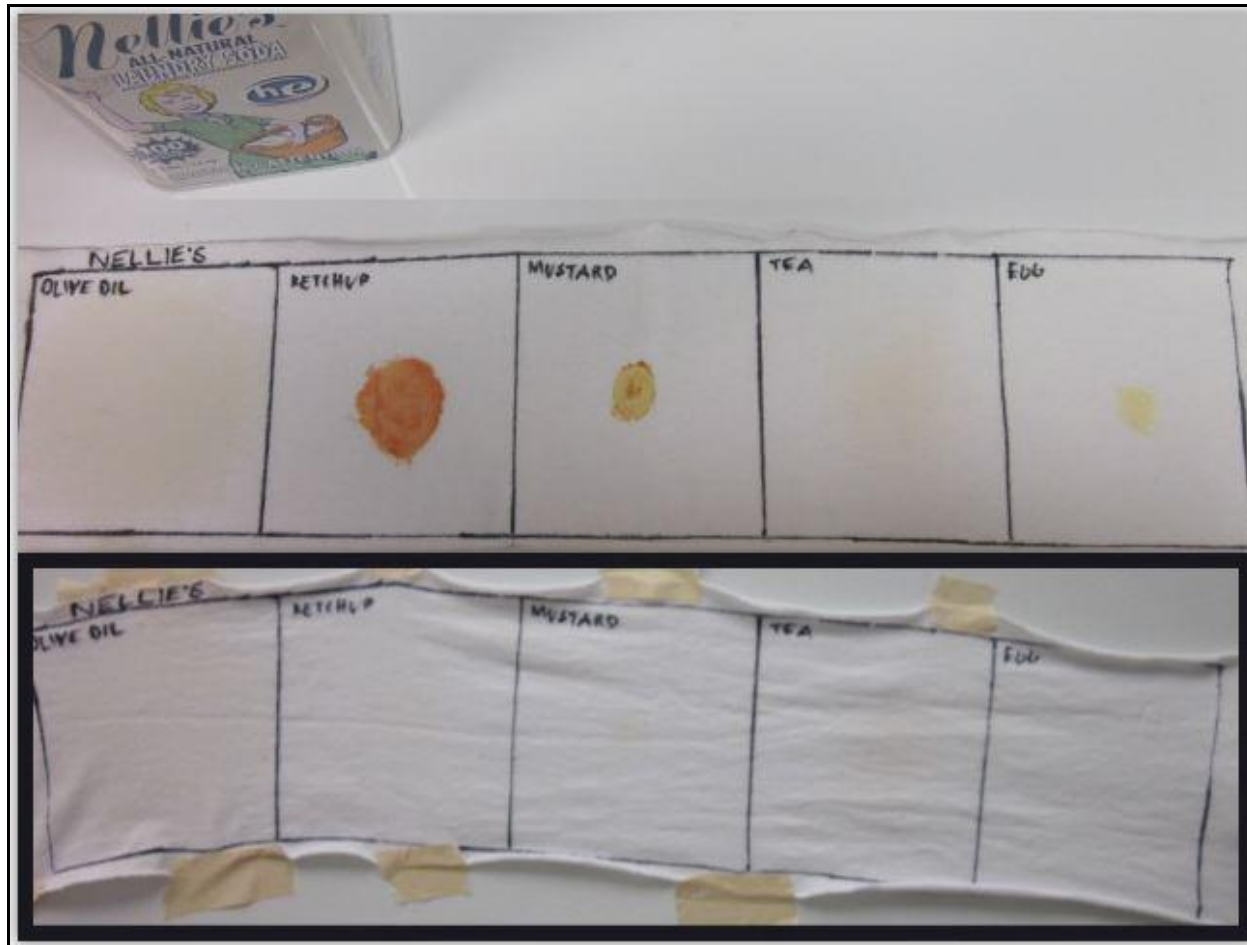
Figure 8. Nellie's before and after performance testing
