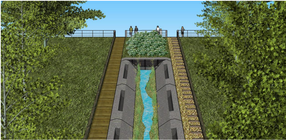
Figure 3 Bio-Retention Stream Bed
