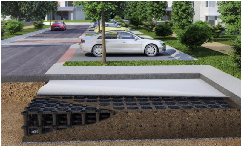
Figure 3. A schematic diagram of a section showing the Silva cells installed underground of the parking lot.
