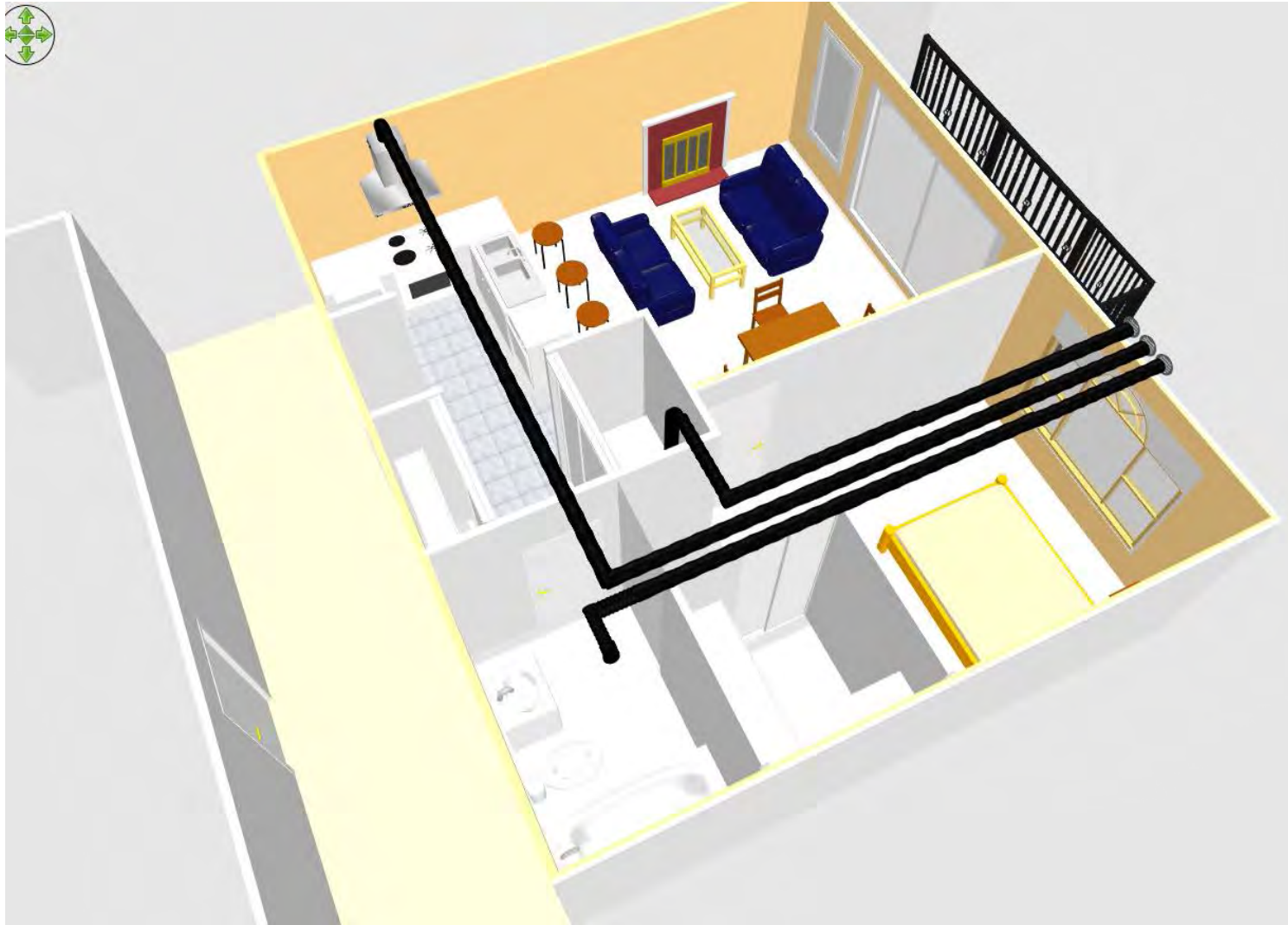
Figure 45 - 1 Bedroom Suite Ducting before HRV Installation
