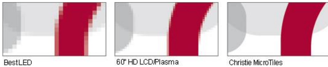
Figure 3: Comparison of Resolution Between Different Screen Technologies
