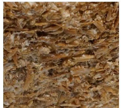
Set #3- Treated Block Visible signs of Cobweb mold contamination about 10% of the surface.
