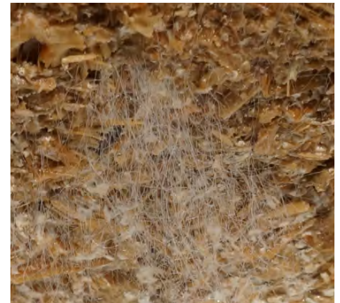
Set #2- Treated Block Visible signs of Cobweb mold contamination about 30% of the surface.
