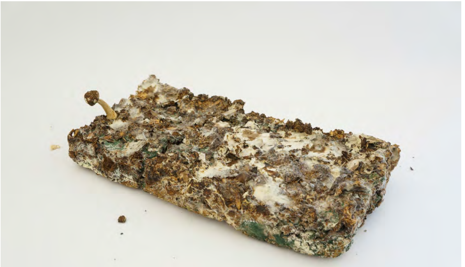
The image above is the day 1 after the putting into the container for moulding. After 7 days of re-colonization, the block is dried for 10 days. There is clear evidence of contamination with molds where the green and black spots are. Shiitake mushroom appears to be more brittle and easy to break even after drying.
