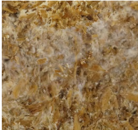
Set #2- GIY Block Most visible signs of fungal colonization. Partial distribution of white coloration.
