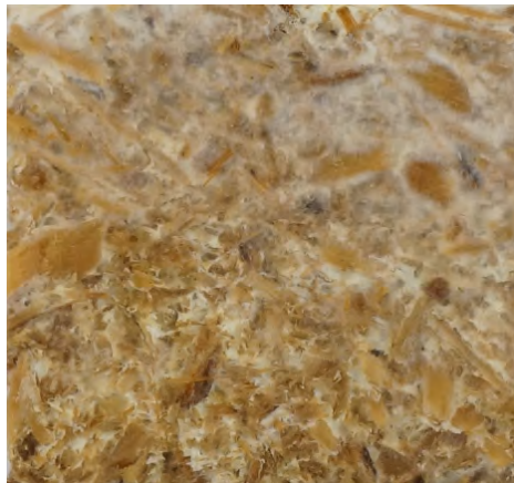
Set #3- GIY Block Some signs of fungal colonization. Partial distribution of white coloration.
