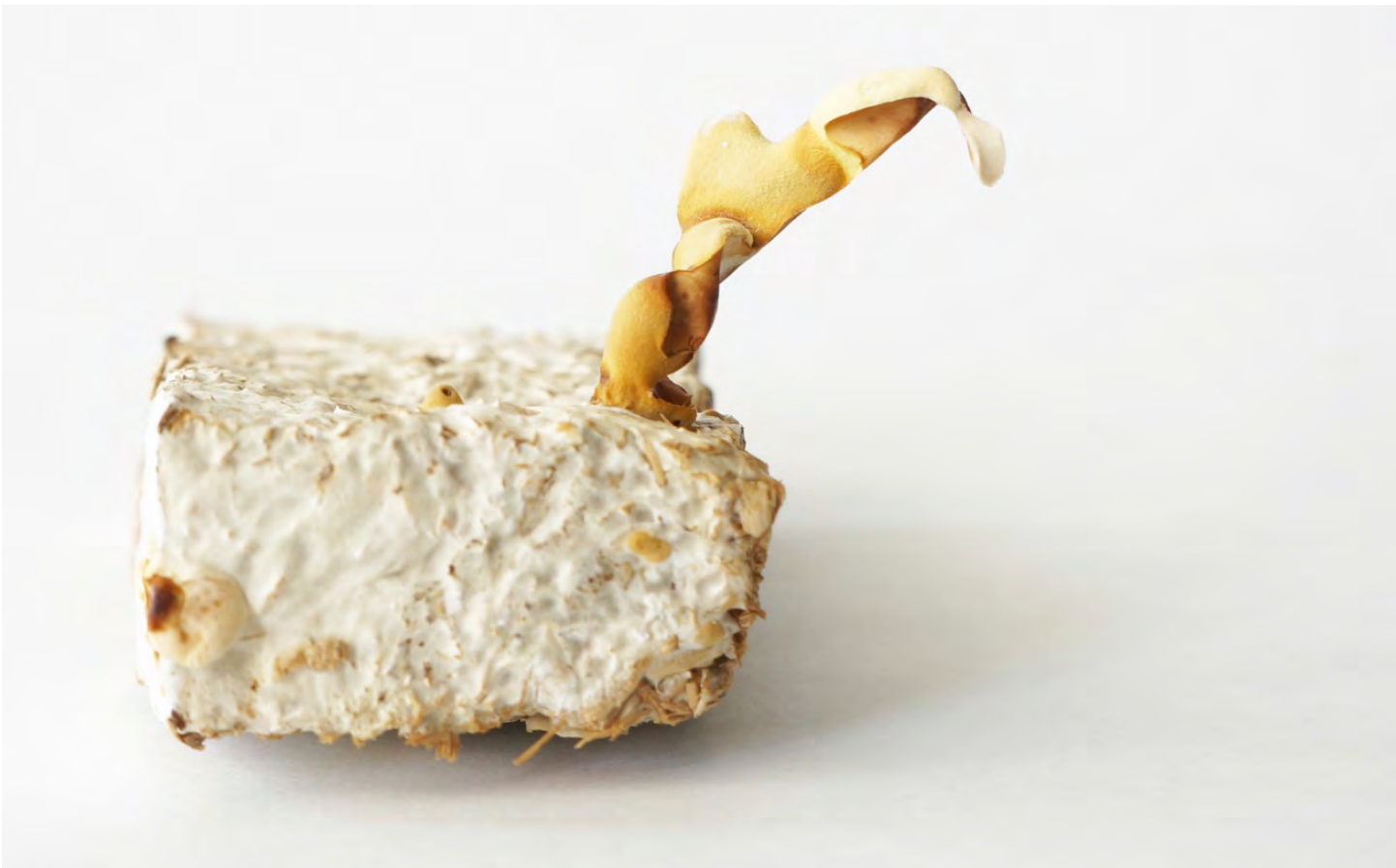
GIY Slice Set #2: Surface Observation after Drying With both GIY Slice set #2 and #3, there is clear shrinkage after a long period of time of drying.
