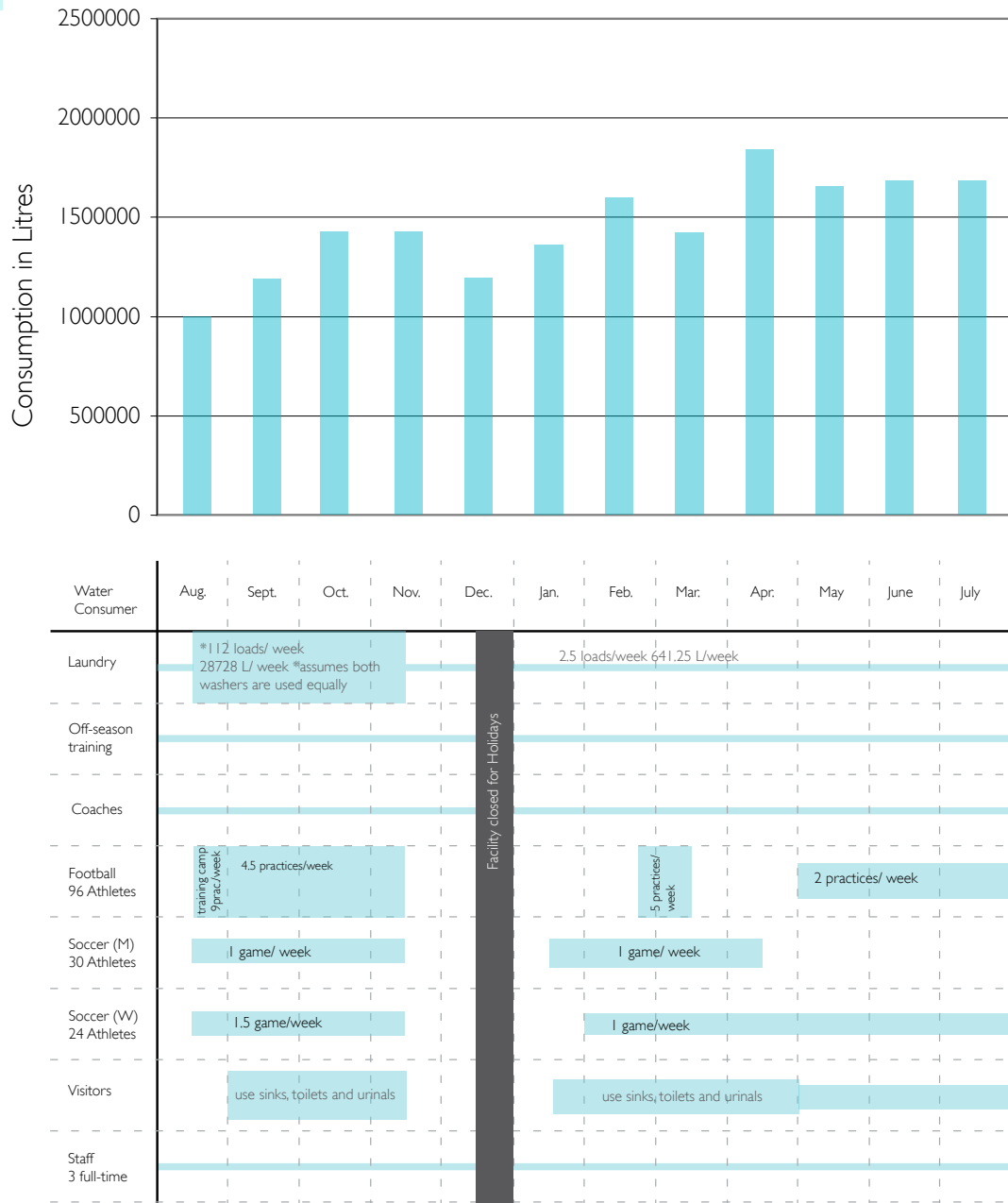
Figure 10. Annual Building Water Consumption with Facility Schedule August 2012- July 2013
