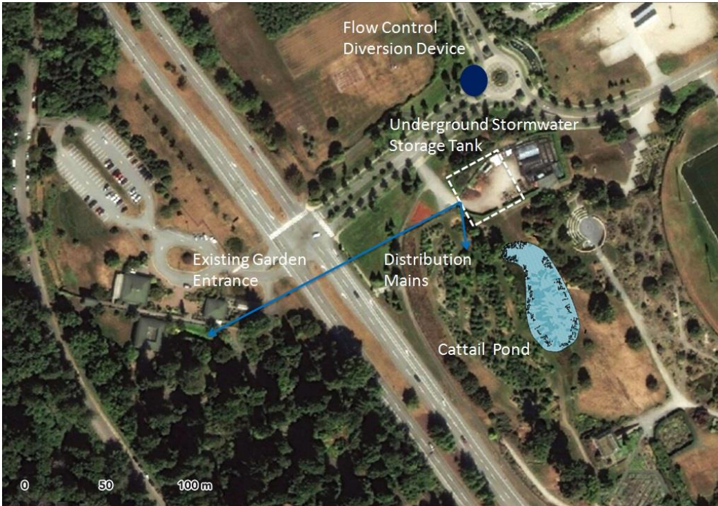
FIGURE 1 AN OVERVIEW MAP OF THE PROPOSED UPGRADES TO THE WATER TREATMENT AND DISTRIBUTION SYSTEM
