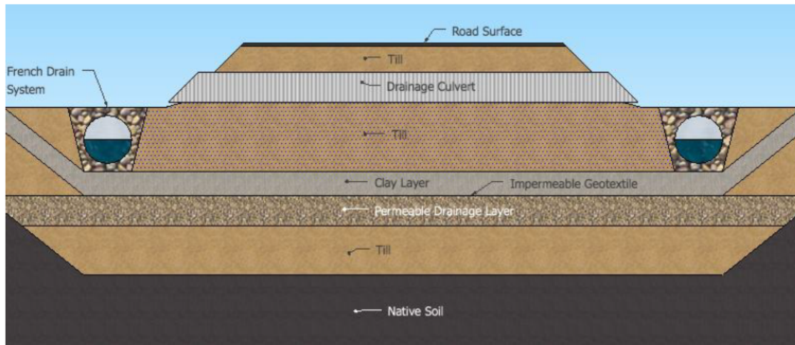
Figure 7. Cross Section of French Drainage System
