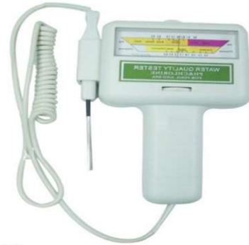
Figure 7-2: Water Quality Testing Device
