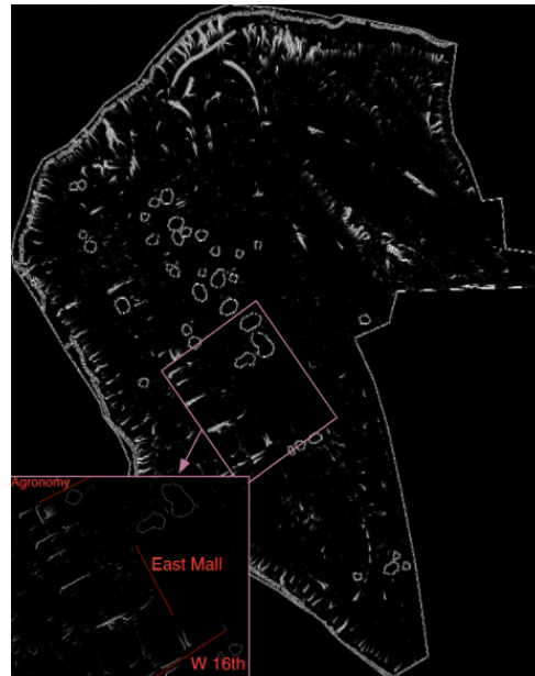
QGIS Flow accumulation model of UBC Campus (Opacity of Whitelines = Density of Flow)
