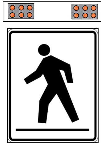
RRFB Pedestrian Crossing
