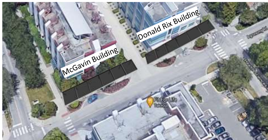
Figure 10: Weathering Canopy Location and Vehicle Access Opening
