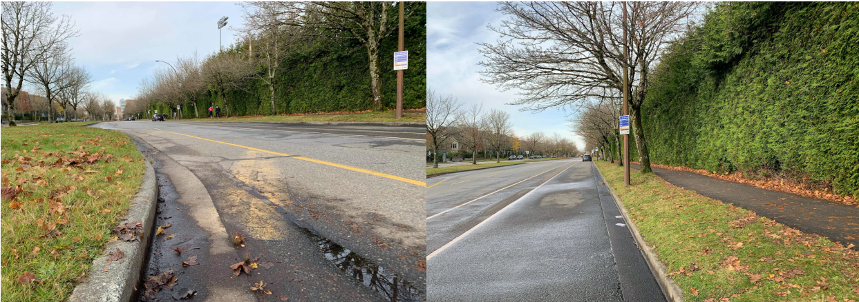
Figure 4: Photos from site visit to East Mall showing parking, painted bike lane (right) and unused space between centre median and travel lane (left)
