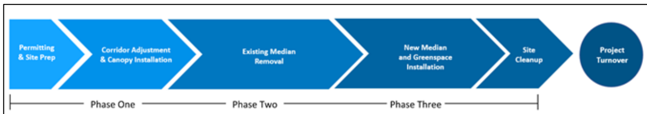
Figure 22: Construction phases and sequencing
