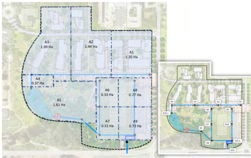
Figure 3 Stormwater Catchment Plan's Drainage Areas
