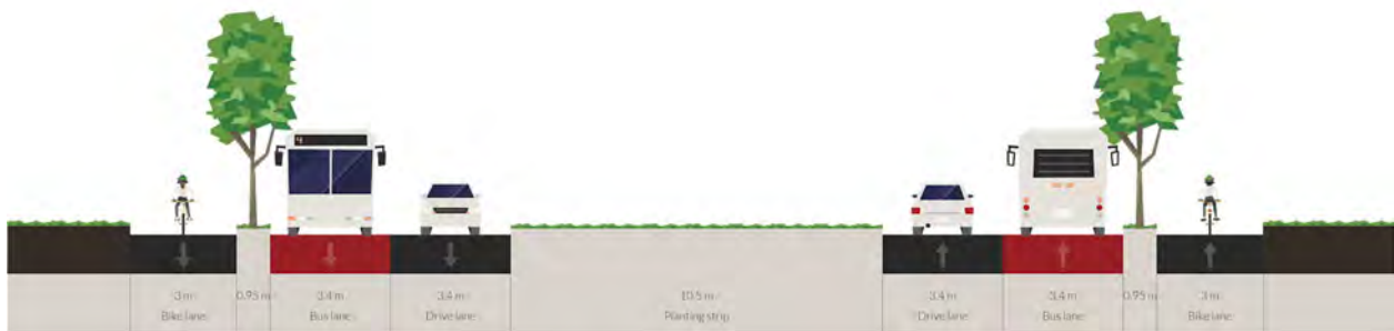
Figure 11 - Proposed W 16th Ave Section View between SW Marine Dr and East Mall
