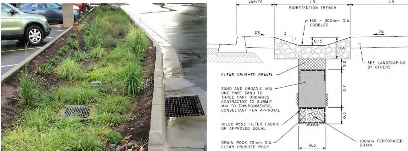
Figure 9 -Typical Bioretention Trench and Cross Section
