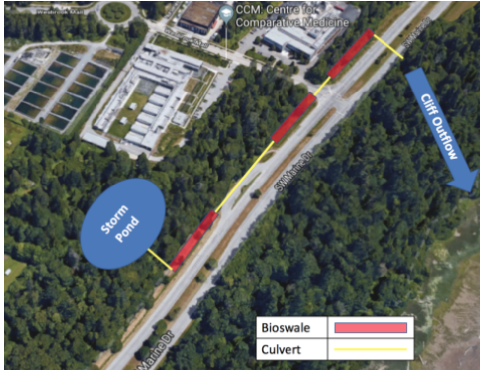
Figure 7: Location of bioswale system along SW Marine Drive.
