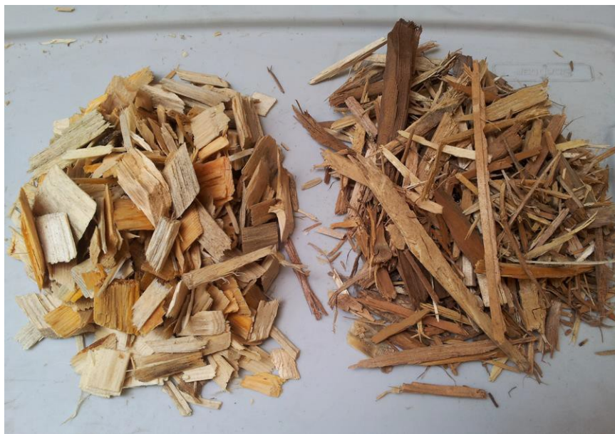
Figure 11. Side by side comparison of wood chips and hog fuel before they are mixed at Cloverdale Fuels Ltd.
