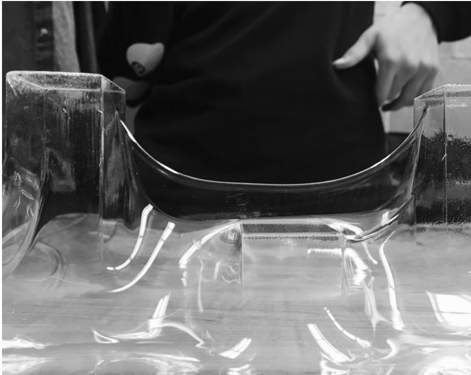
Early tests included using different plastics, shapes and temperatures to achieve lofted forms and complex curves.
