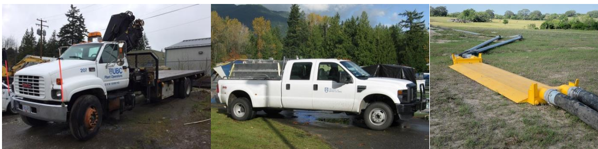
Figure 6 Transportation alternatives considered. From left to right: flatbed truck with crane to which an auto-levelling attachment could be attached (Francois Desmarais), pickup truck which would tow trailers with water buffalo (Carleton University, n.d.), piping (with road crossing pictured) (TanMar Companies, n.d.).
