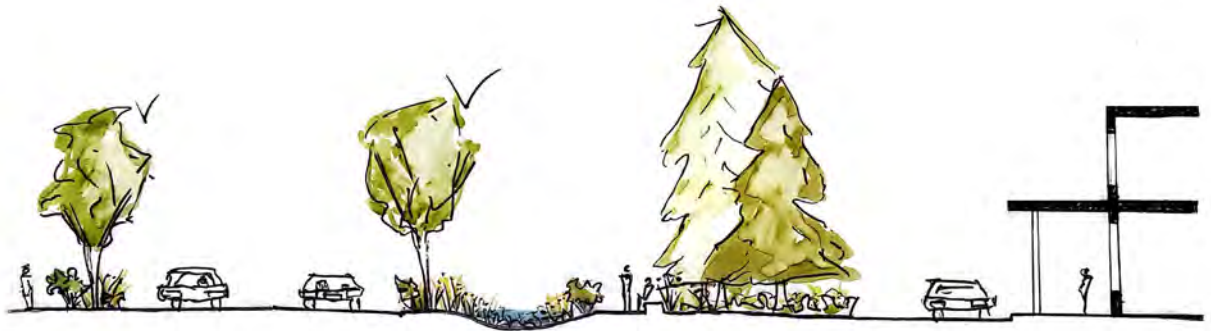
Section - Wesbrook Mall and Swales facing south
