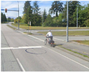
UNBUFFERED BIKING LANE ALONG ARTERIAL DRIVEWAYS
