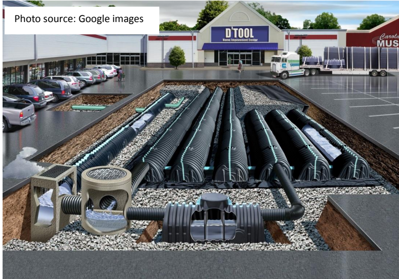
Figure 5: Subsurface stormwater collection system
