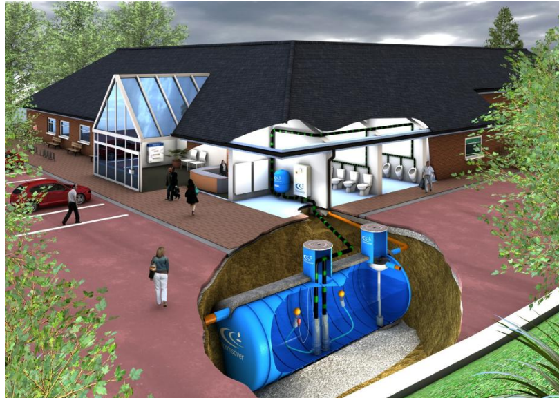
Figure 15 -Rainwater Collection and Storage (Stormsaver, 2013)
