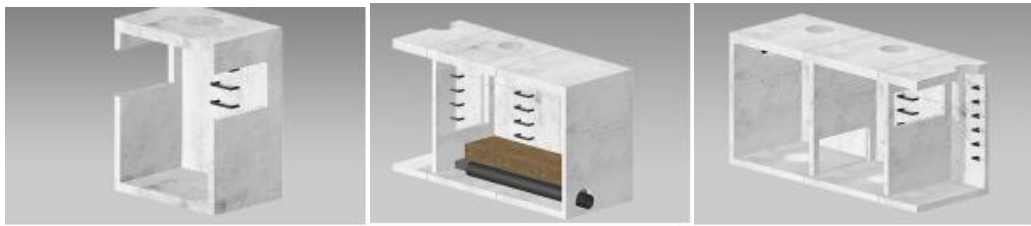
Figure 15: From left to right - sedimentation module, filtration module, and Oil/water separation module
