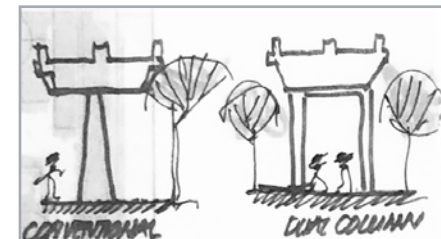
Conventional Vancouver guideways support structure vs. dual column structure for provision of public space.
