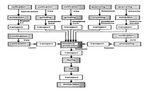
Figure 2: Flowchart of the Life-Span of Linoleum Adapted: Jonsson, Tillman, Svensson, 1996, p. 247
