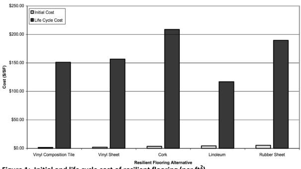
Figure 1: Initial and life cycle cost of resilient flooring (per ft<sup>2</sup>) Adapted: Moussatche et al., 2001, p. 336
