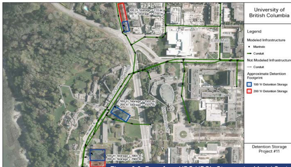
Figure 3.8: Page from UBC UBC's Stormwater Model System Analysis, Detention Analysis and System Optimization study indicating the location and size of detention tanks required to handle surplus water (GeoAdvice Engineering Inc., 2013).
