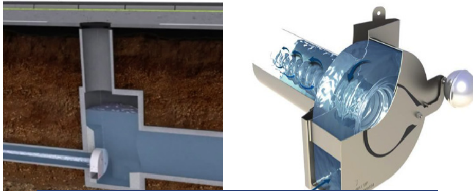
Figure 3.9: Left: Schematic of a flow management device in operation (Hydro International, 2016). Right: The Hydro-Brake Optimum, a vortex flow control device from the UK (ACO, 2010).
