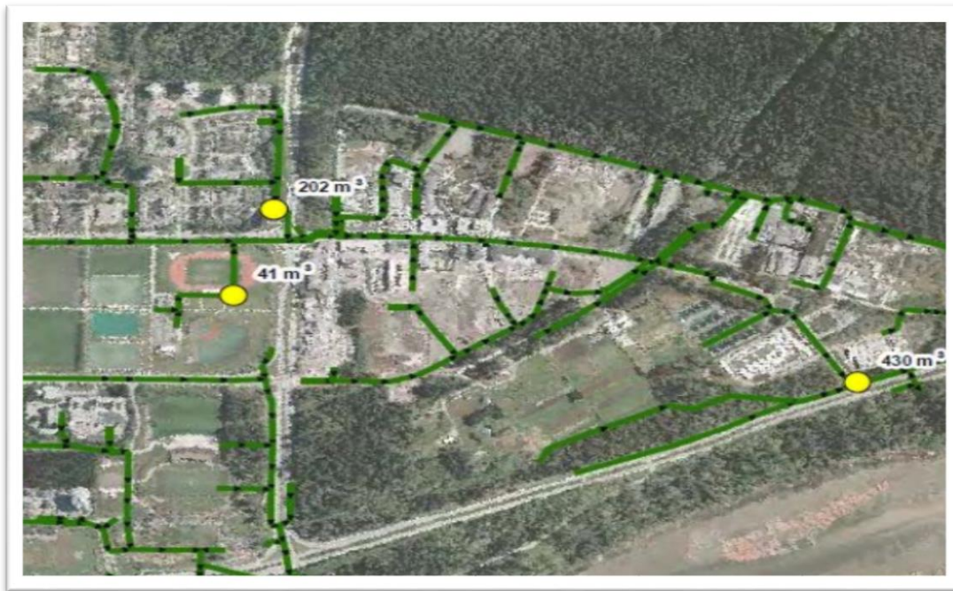
Figure 4 Flooding Issues during 10-Year Storm Event
