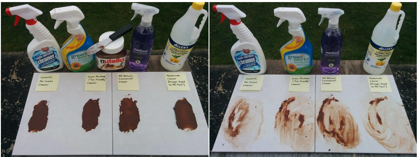
Figure 5: Before (left) and After (right) photos of cleaner performance test
