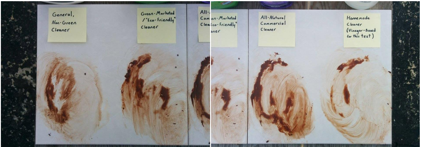
Figure 6: After photos of cleaner performance test in close-up
