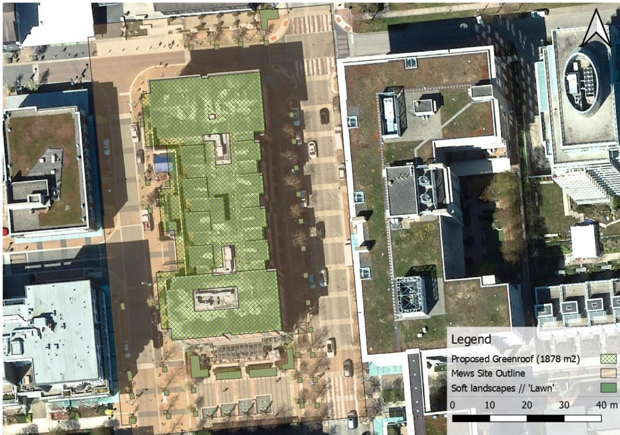
Figure 4 - A close-up of The Mews, in close proximity to University Hill Secondary School and Westbrook Community Centre (just to the hypothetical left of the image above). The map above displays the theoretical plots that could cover the roof surface whilst avoiding machinery, as well as shapes from the Softlandscape analysis by Nicholas Mantegna.
