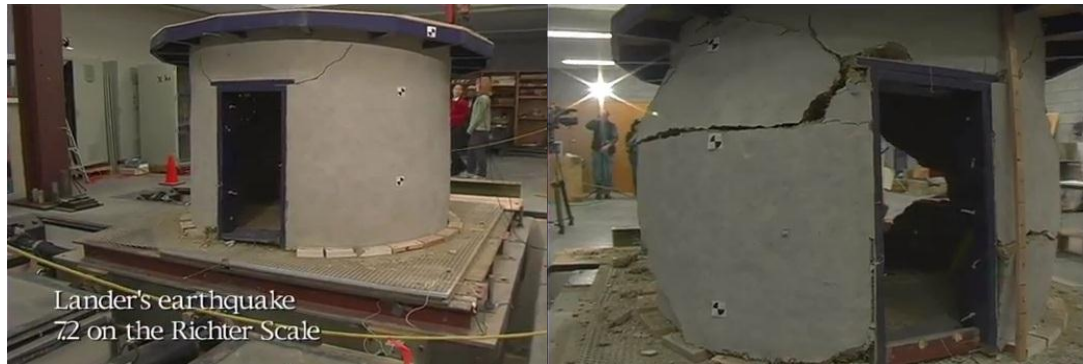
Figure 3: Stanley Park Ecology Society simulates a 7.2 (Left) and 9.0 (Right) earthquake on a cob structure at the UBC Earthquake Engineering Research Facility
