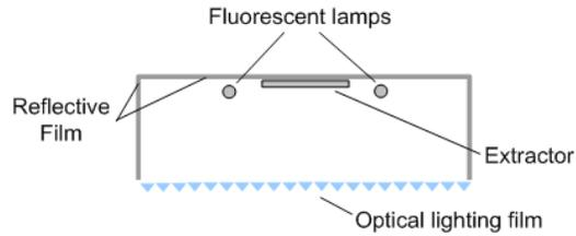
*Figure 2 – Cross Section of the Light Pipe (1)*
